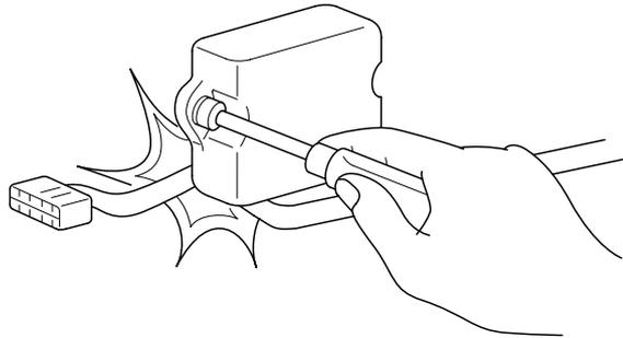
6. The electronic parts used in the computer, relays, etc. are readily damaged by heat. If there is a need for service operations that may cause the temperature to exceed 80°C (176°F), remove the electronic parts before hand.
