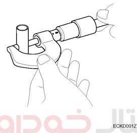
2. Check the piston pin-to-piston clearance.
