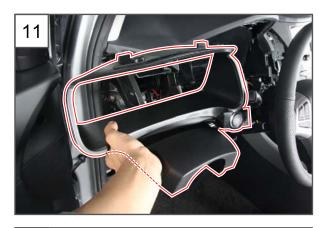
11.Remove the instrument cluster fascia panel assembly.
