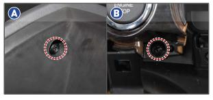
10.Detach the instrument cluster fascia panel assembly to disconnect the START/STOP switch connector.
