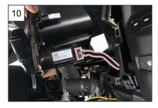
Unscrew the mounting screws (two for A, one for B) on the instrument cluster fascia panel assembly.
