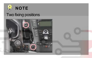
5. Unscrew the two LH side fascia panel mounting screws.
