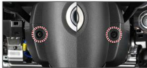
8. Unscrew the one shroud lower cover mounting screw (A), lower the column tilting lever and remove the shroud lower cover.
