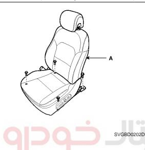
3. Disconnect the power seat (A) and airbag (B) connectors.
