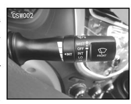
Use the operating lever on right side of steering column to operate the front windshield wiper.
