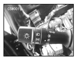
To deliver a change lane signal, push the operating lever up or down till the end. When the turn is finished, the operating lever will automatically retract. There are two flashing arrows on the combination instrument, which display the turn direction signals.
