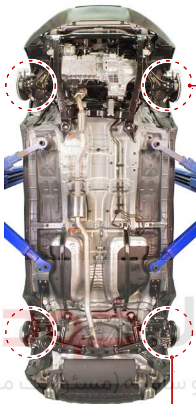
Rear wheel speed sensor for 2WD
