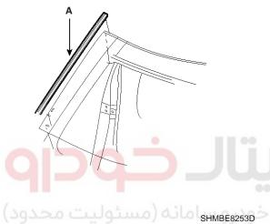
3. Cut out the windshield sealant using the sealant cutting tool (A)(09861-31100).
