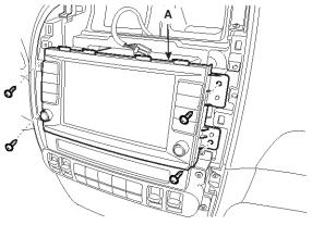
6. After loosening the heater control mounting screws, remove the heater control unit (A).
