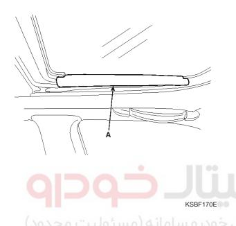
2. Remove the glass (A) by lifting it up.
