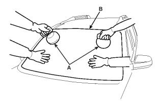
4. Remove the windshield (A) carefully using the glass
