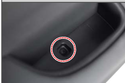
A. Armrest panel Mounting screw
