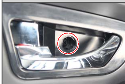
B. Inside handle Mounting screw
