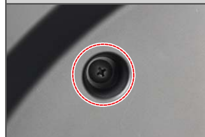
C. Door trim right side upper mounting screw
