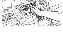
Check airbag inflator case for dents, cracks or deformities.
