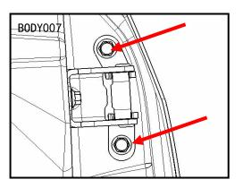
■ Tightening torque: 16.7~25.5 N.m
