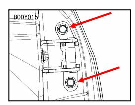
■ Tightening torque: 16.7~25.5 N.m
