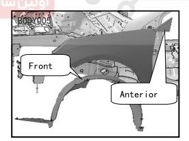
④ Use No. 10. socket of 6 angles to remove 8 combination bolts in the fender.
