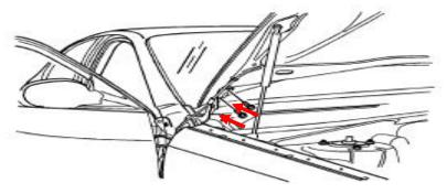
Tightening torque: 9~11 N.m, 16.7~25.5N.m
