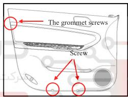
5 Use a slotted screwdriver to pry up the 8 buckles on the front door interior trim panel,
