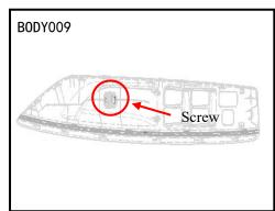
panel and door trim assembly, remove the armrest panel, and disconnect the connector of the switch assembly
