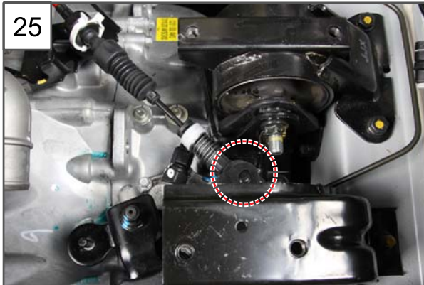
25. Disengage the transaxle selector cable link rod.
