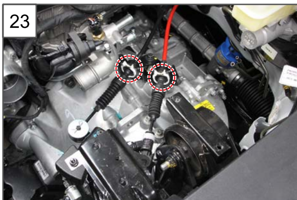
23.Remove the transaxle cable holder.
