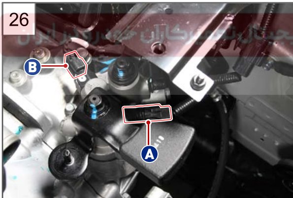
26. Disconnect the transaxle switch connector (A) and the backup lamp switch connector (B).
