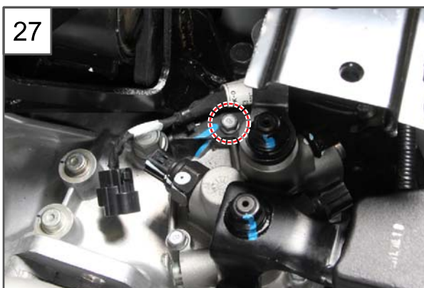
27. Unscrew the bolt (10 mm) and remove the connector bracket.
