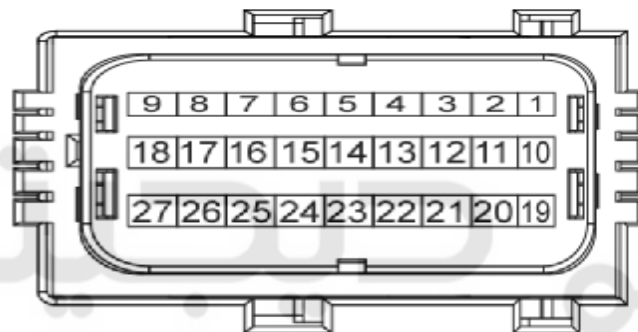
M60-A SRS Control Module - 27 Female / Green (AMP_ACU_27F_Curry)
