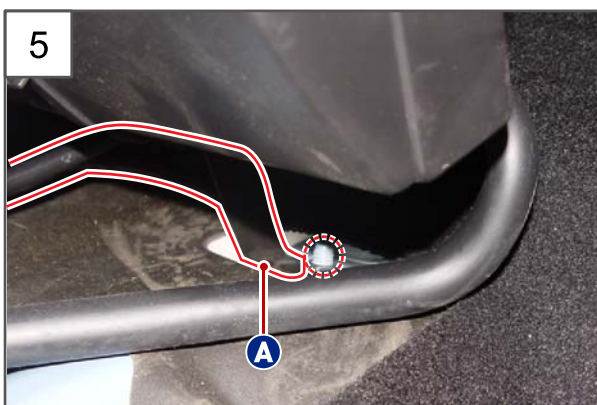
Press the shift cable mounting clip to the arrow direction.
