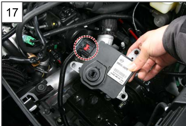
17. Disconnect the TCU wiring connector.
