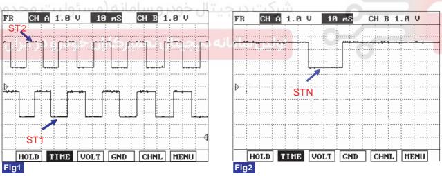
Fig 1) Test Condition : Ignition "ON" & Engine "ON". Normal data ( Approx. High : 3.5V , Low : 1.5V )
