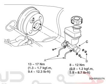
Remove the master cylinder (C) from the brake booster. Be careful not to bend or damage the brake lines when removing the master cylinder.
