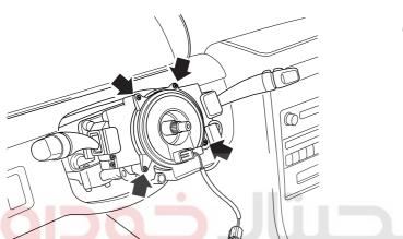
Tighten two bolts after installing the air module.
