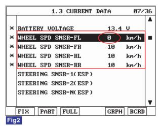
Fig 1) Test Condition: Drive vehicle at a speed of 10km/h or more. (6.2mph or more) Normal Data
