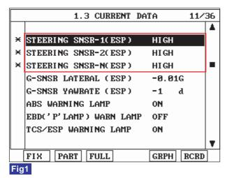
Fig 1) Test Condition : Ignition "ON" & Engine "ON".
