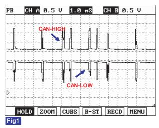
Fig 1) Normal Waveform with Ignition "ON".
