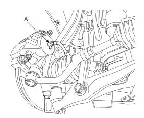
Install the brake hose clip (A) to the brake hose bracket.
