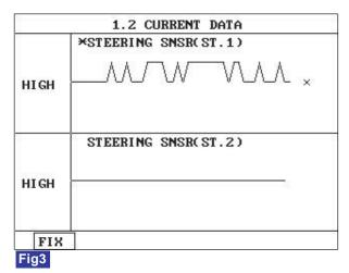
Fig 1) Test Condition: Ignition "ON" & Engine "ON". Normal data Fig 2) Test Condition: Ignition "ON" & Engine "ON". Normal graph Fig 3) Test Condition: Ignition "ON" & Engine "ON". Abnormal graph
