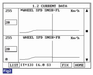
Fig 1) Test Condition: Drive vehicle at a speed of 20km/h or more. (12.4mph or more) Normal Data Fig 2) Test Condition: Drive vehicle at a speed of 20km/h or more. (12.4mph or more) Normal Graph
