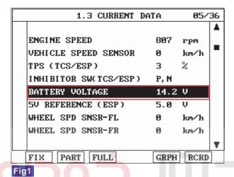
Fig 1) Test Condition : Ignition "ON" & Engine "ON".
