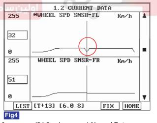
Fig 1) Test Condition : Drive vehicle at a speed of 40km/h or more. (24.9mph or more) Normal Data
