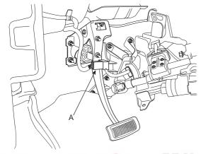
Remove the adjustable cable (A) in case of the adjustable brake pedal.
