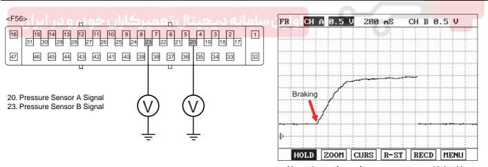
Normal waveform of pressure sensor with braking
