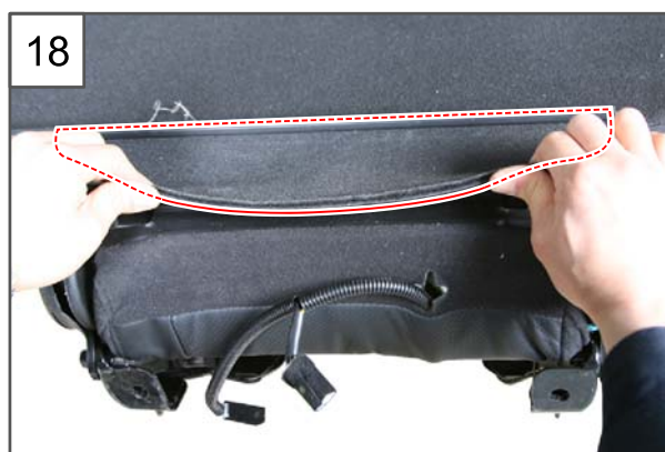
18.Remove the rear seat lower cover of the 1st row.
