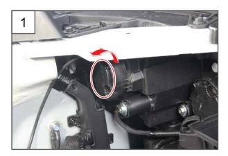
1. Turn the low beam cap to the arrow direction behind the headlamp assembly to remove it.
