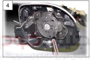
4. Separate the puddle lamp from the outside rearview mirror housing using a flat-bladed screwdriver.
