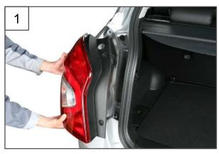
1. Disconnect the rear combination lamp assembly.
