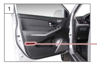
1. Remove the door courtesy lamp lens using a flat-bladed screwdriver or equivalent.
