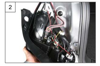
2. Disconnect the rear combination lamp connector.
