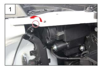
1. In order to remove the turn signal lamp bulb and socket, turn those parts to the arrow direction behind the headlamp assembly.
