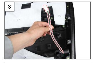
3. Remove the door courtesy lamp assembly.
