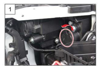
1. Turn the high beam cap to the arrow direction behind the headlamp assembly to remove it.
