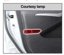
The door courtesy lamp comes on when the driver's door or passenger's door is opened.
