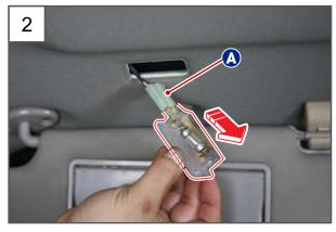
2. Disconnect the sun visor lamp connector (A) and remove the sun visor lamp.
