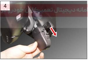
4. Pull out the AUTO light sensor module to the arrow direction.
