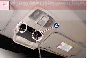
1. Unscrew the 2 mounting bolts (10 mm) on the overhead console.
