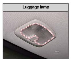
The luggage lamp is turned on when the tailgate is opened with the switch operated.
