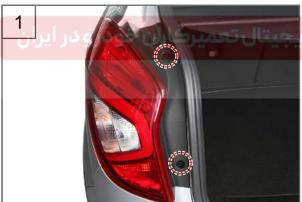
1. Unscrew the 2 mounting screws for the rear combination lamp.
