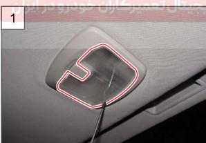
1. Remove the lamp cover using a flat-bladed screwdriver.
