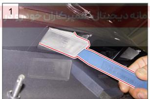
1. Remove the inner side (clip part) of the license lamp first carefully from the tailgate rear garnish.
