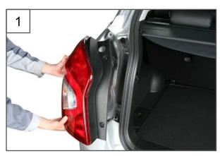
1. Disconnect the rear combination lamp assembly.
