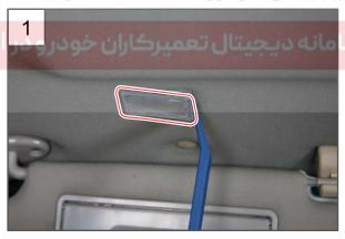
1. Separate the sun visor lamp assembly from the headlining using a flat-bladed screwdriver.
