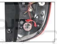
3. Turn the stop lamp bulb to the arrow direction to remove it.
