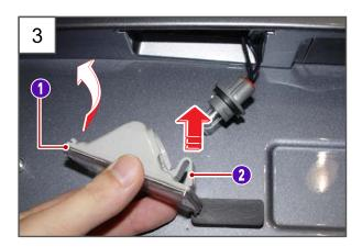
3. Always engage the hook part (1) first and press the clip part (2) with the bulb fitted.
