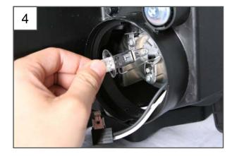
4. Remove the high beam bulb.
