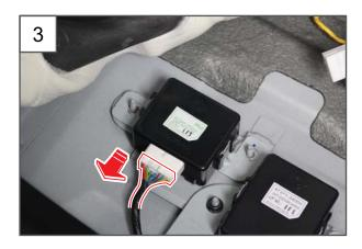
3. Disconnect the connector and remove the DRL unit.
