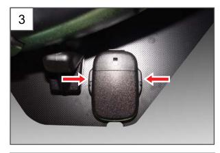
Insert the screwdriver into the service holes at both sides of the cover to separate between the upper and lower covers.
