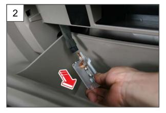
2. Disconnect the connector and remove the glove box lamp.
