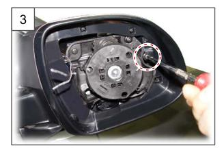
3. Remove the one turn signal lamp mounting screw from the outside rearview mirror.
