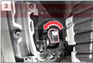
3. Turn the fog lamp bulb to the arrow direction to remove it.
