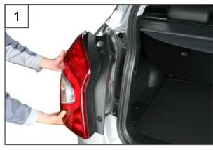
1. Disconnect the rear combination lamp assembly.
