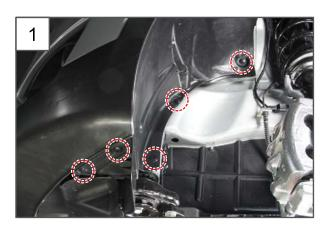
1. Remove the 5 screw rivets securing the front wheel house cover.
