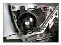
4. Remove the front fog lamp assembly.
