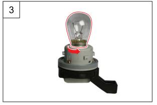
3. Remove the turn signal lamp bulb from the socket while pressing it downwards.
