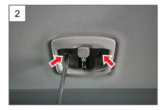
2. Remove the 2 room lamp mounting nuts (10 mm)
