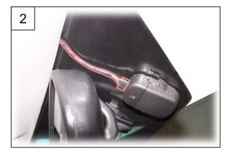
2. Disconnect the connector from the AUTO light & rain sensor module.
