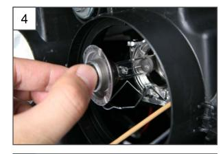
4. Remove the low beam bulb.
