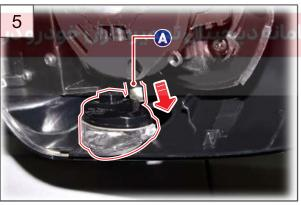
5. Disconnect the puddle lamp connector (A) and remove the puddle lamp.
