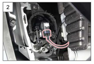
2. Separate the wheel house cover and disconnect the front fog lamp assembly.
