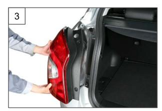
3. Disconnect the rear combination lamp assembly.
