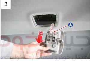
3. Disconnect the room lamp connector (A) and remove the room lamp assembly.
