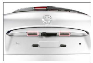
When the corresponding lamp comes on and goes off by operating the tail lamp, AUTO light, high beam and low beam on the multifunction switch, the license lamp also does.
